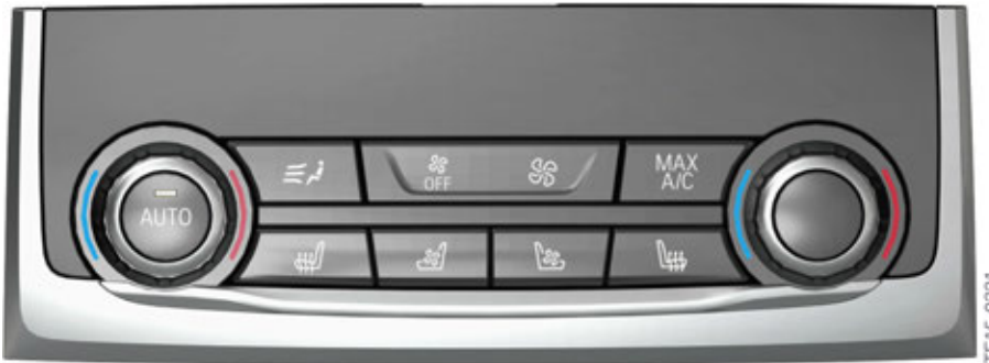
G12 4-zone IHKA control panel for rear passenger compartment
